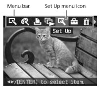
To exit the menu mode, press MENU. The previous window is displayed. 2 Press ⊲/⊳ to select (Set Up) and then press ENTER. The Set Up menu is displayed.
